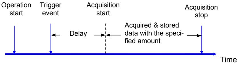
**Figure 4.6 Delay trigger**
