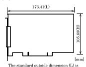
the distance from the end of the board to the outer surface of the slot cover.
