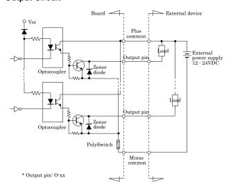
The output circuit of interface is illustrated in the above Figure. The signal output section is an opto-coupler isolated, open-collector output (current sink type). Driving the output section requires an external power supply. The rated output current per channel is 100 mA at maximum.
