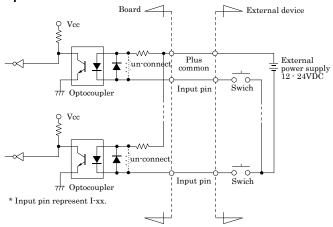
The input circuit of interface is illustrated in the above Figure. The circuit is connected to a device that can be current-driven, such as a switch or transistor output device.
