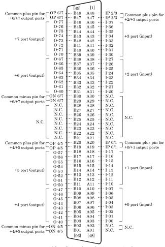
\* I-00 - I-37 can be used as interrupt signal. The numbers in square brackets [] are pin numbers designated by
