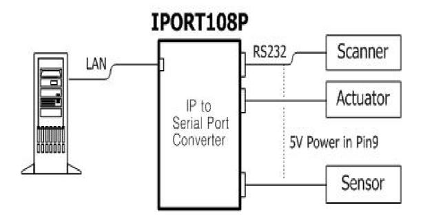
This is one structure for test equipment used in iPhone 7's production work line. And you can have similar structure in your next application environment. IPORT108P box is your solution.
