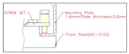
by releasing thumb-screw and turn 90deg, then tighten toward the mounting panel.
