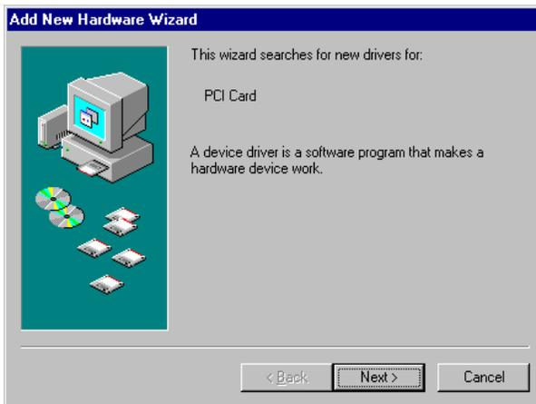
You can click **Next** button to go on installing device. The device information files are located in "DASK98Inf" directory of **ADLink All-in-**
