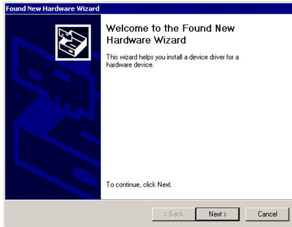
You can click **Next** button to go on installing device. The device information files are located in "DASK2000Inf" directory of *ADLink All-in-One CD*. However the device cannot work properly without the software
