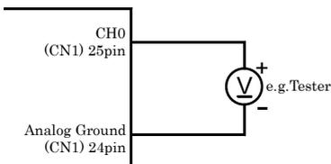
Figure 2.4. Connection diagram
