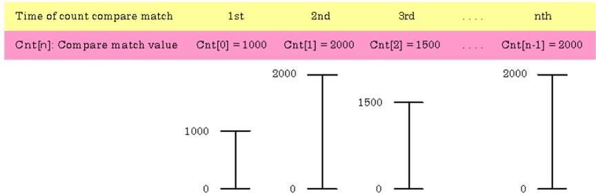
The figure above shows an example of using the compare count load function.
