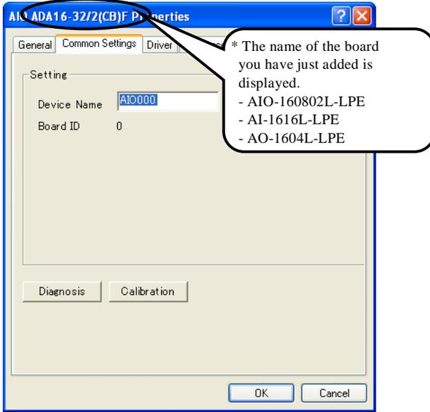
Proceed with connecting the calibration equipment and performing the calibration in accordance with the instructions displayed by the calibration program.
