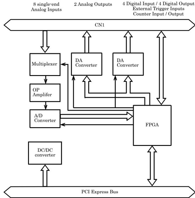
Figure 6.1. Block Diagram < AIO-160802L-LPE >
