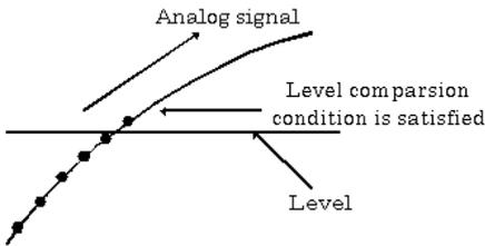
The above sketch shows that the level comparison condition is satisfied in the rising direction. The stop condition is satisfied when the analog signal at the specified channel passes the comparison level in the rising direction. Input data items are stored to memory, ending until those at solid dots.
