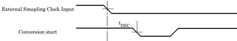
**Figure 6.4. Timing Chart of External Smampling Clock**
