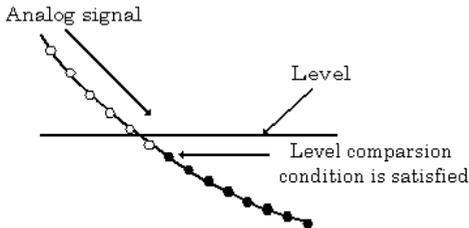
The above sketch shows that the level comparison condition is satisfied in the falling direction. The start condition is satisfied when the analog signal at the specified channel passes the comparison level in the falling direction. Input data items are stored to memory, starting with those at solid dots.
