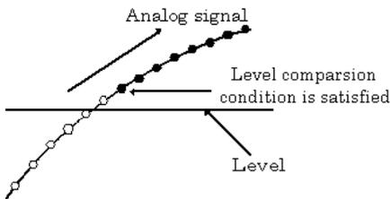
The above sketch shows that the level comparison condition is satisfied in the rising direction. The start condition is satisfied when the analog signal at the specified channel passes the comparison level in the rising direction. Input data items are stored to memory, starting with those at solid dots.
