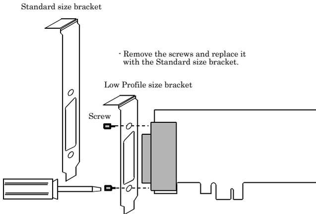
Use a flathead screwdriver or hexagonal spanner to undo and tighten the screws.
