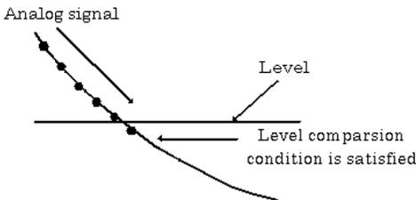
The above sketch shows that the level comparison condition is satisfied in the falling direction. The stop condition is satisfied when the analog signal at the specified channel passes the comparison level in the falling direction. Input data items are stored to memory, ending until those at solid dots
