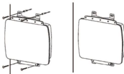
Instead of screwing the screws in all the way, it is advised to leave a space of about 2mm to allow room for sliding the device between the wall and the screws.
