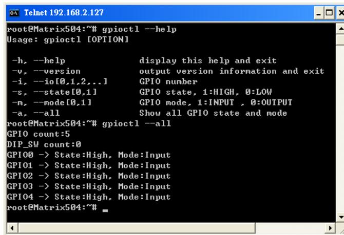
A terminal window titled "Telnet 192.168.2.127" showing the execution of the gpioctl command. The user enters "gpioctl --help" and the terminal displays the usage information for the command. The user then enters "gpioctl --all" and the terminal displays the state and mode for GPIO pins 0 through 4.
