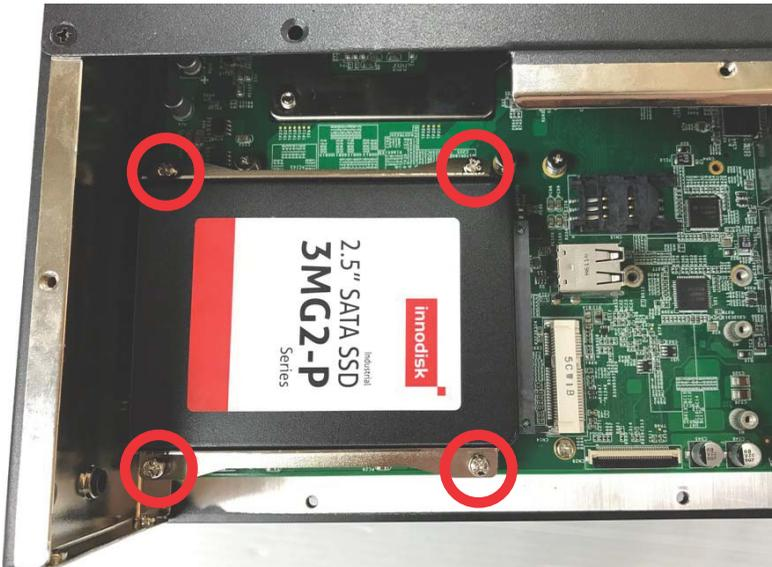
6. Replace the bottom cover and refasten screws.
