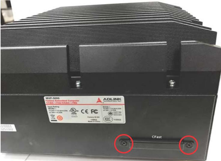
2. True the CFast card with the alignment guide.
