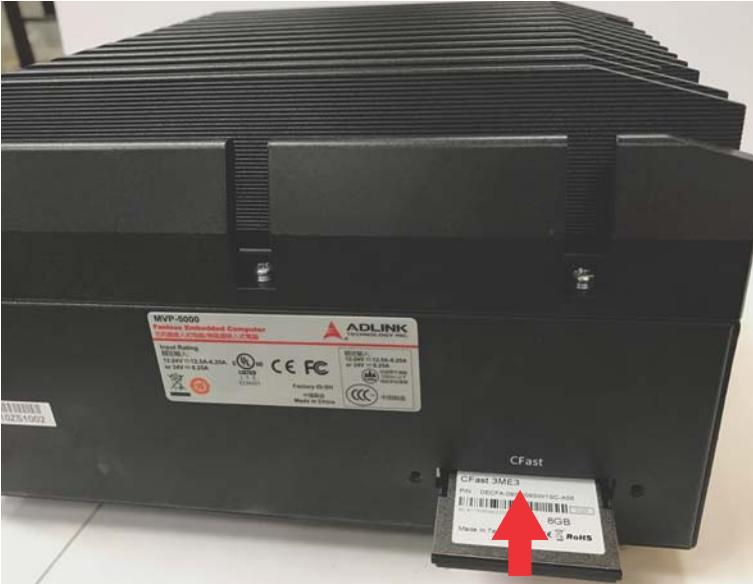
3. Gently insert the CFast card until it is firmly seated in the socket.
