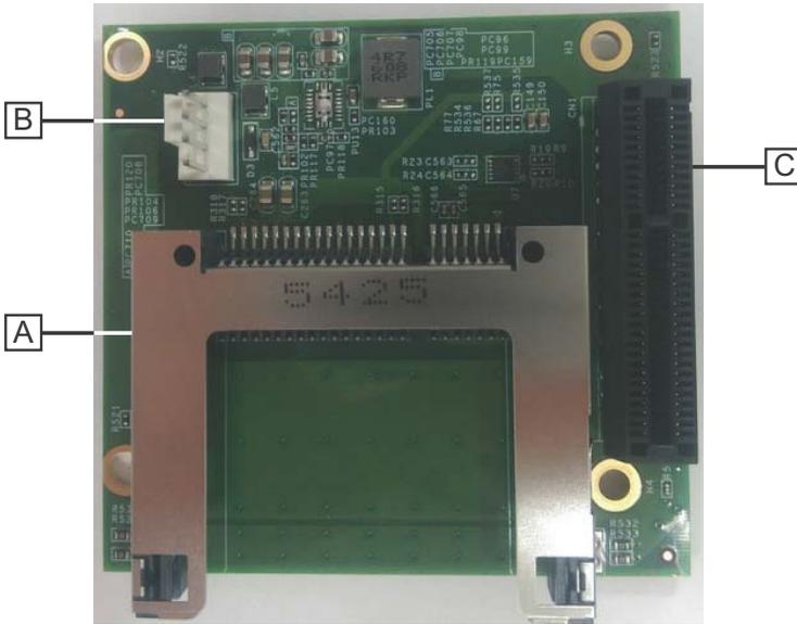
**Figure 1-19: CFast Board Connectors**
