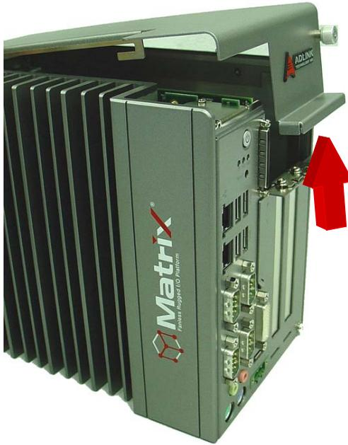
3. Remove 2 screws from the top of the HDD bracket.
