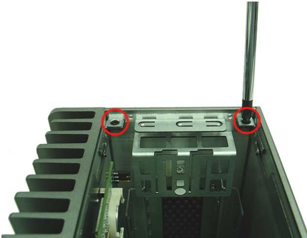
4. Place the chassis upside down and remove the other 2 screws from the bottom of the HDD bracket..
