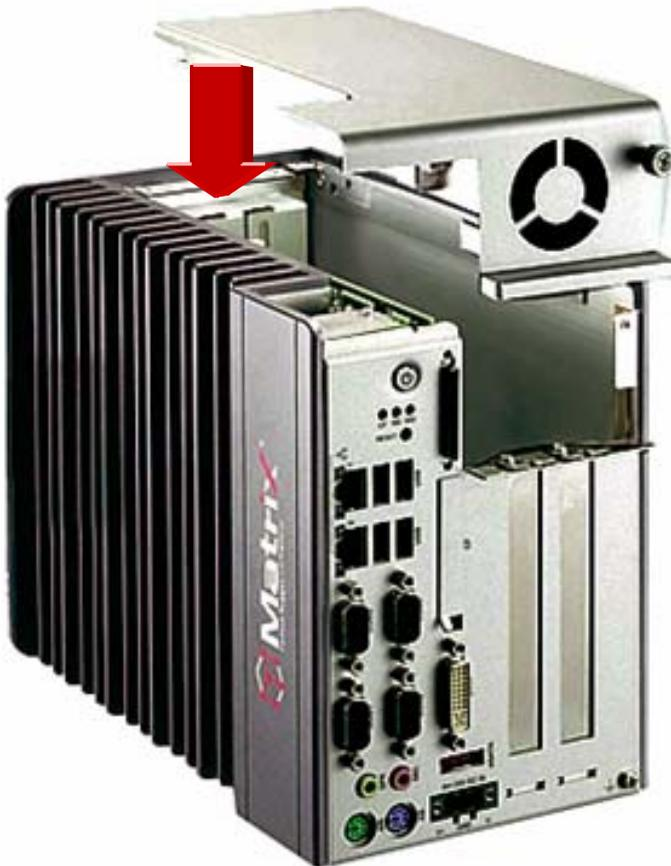
2. Slide the fan module back until USB connection is secured, as shown.
