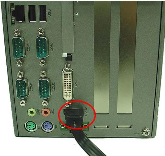
2. Connect the eSATA cable and a DC power supply to an
