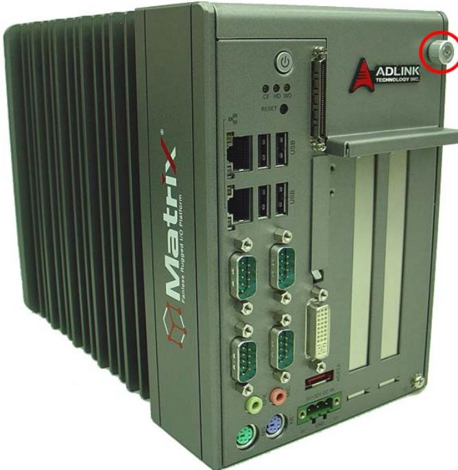
2. Withdraw the thumbscrew and remove the top cover by lifting.
