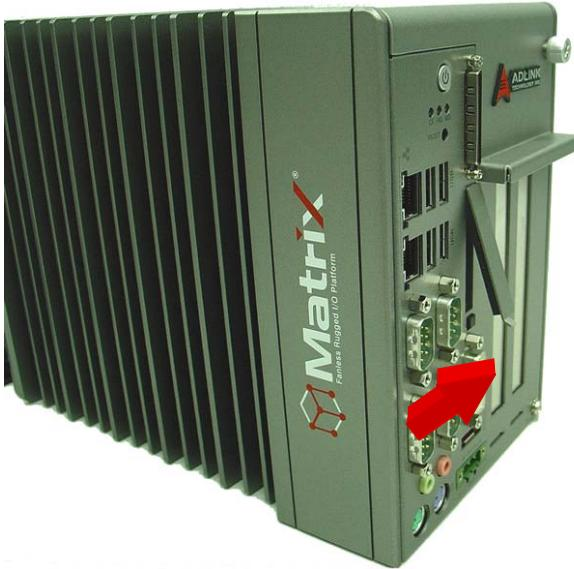
6. Align the externally mounted CF card with the guide of the external CF socket.
