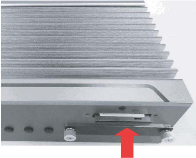
3. Replace the CFast cover and refasten the 2 screws.
