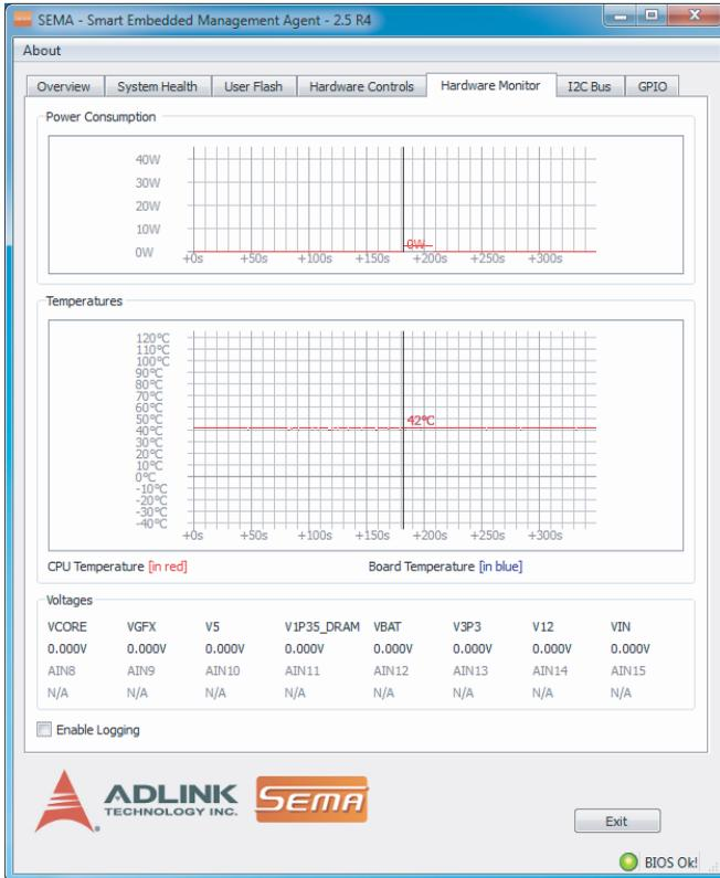
When logging is enabled, all values queried every second, such as temperatures and power consumption, are recorded to a log file.
