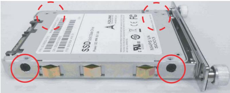
5. Gently slide the bracket back into the bay until the SATA connector on the PCB is engaged.
