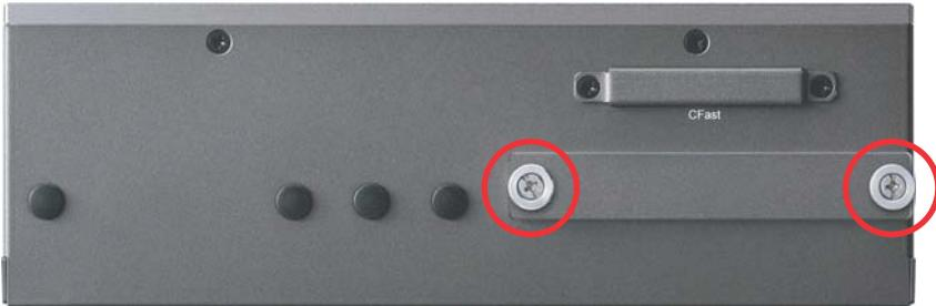
2. Withdraw the HDD bracket.
