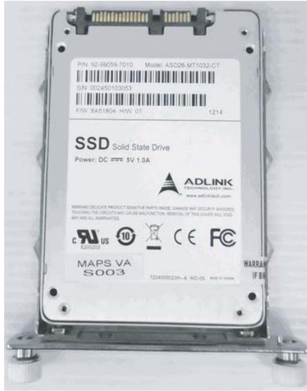
4. Use the 4 provided M3 screws to fix the unit to the bracket.
