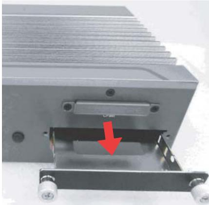
3. Place the HDD or SSD into the bracket.
