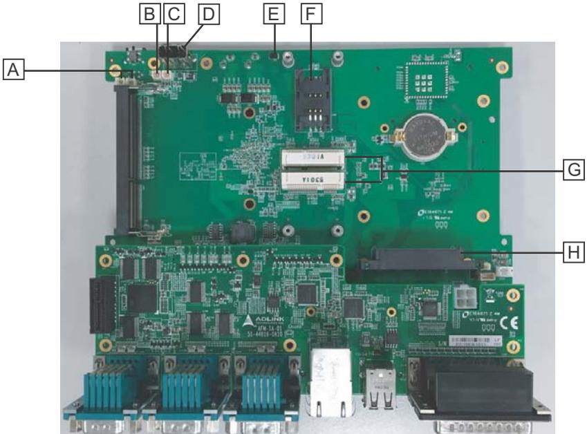
**Figure 1-14: Internal I/O**
