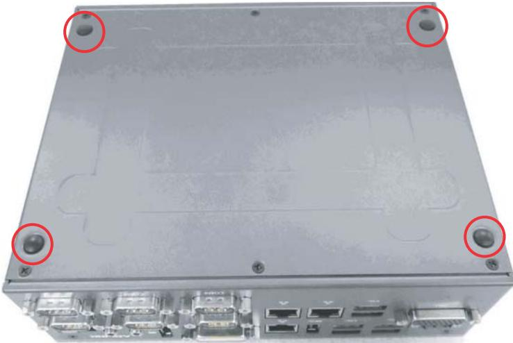
2. Use the 4 M4 screws shipped with the controller to fix the 2 wall-mount brackets, also included, to the chassis, according to the spacing dimensions of the screw holes and brackets, as shown.
