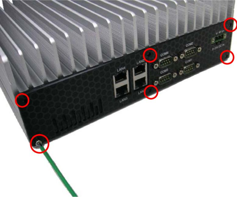
3. Turn the system upside down and lift the chassis..
