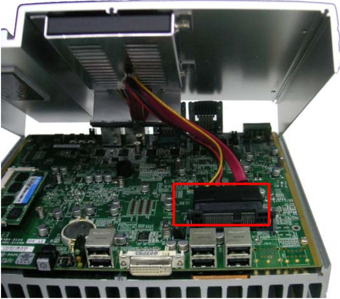
4. Unplug the SATA cable from the SATA connector (receptacle) on the PCB..
