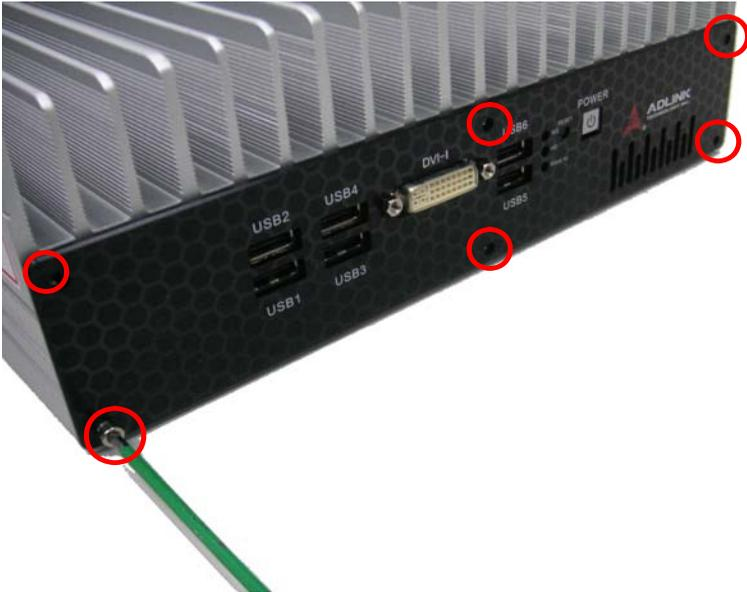
2. Remove the 6 screws from the rear panel and remove the panel.
