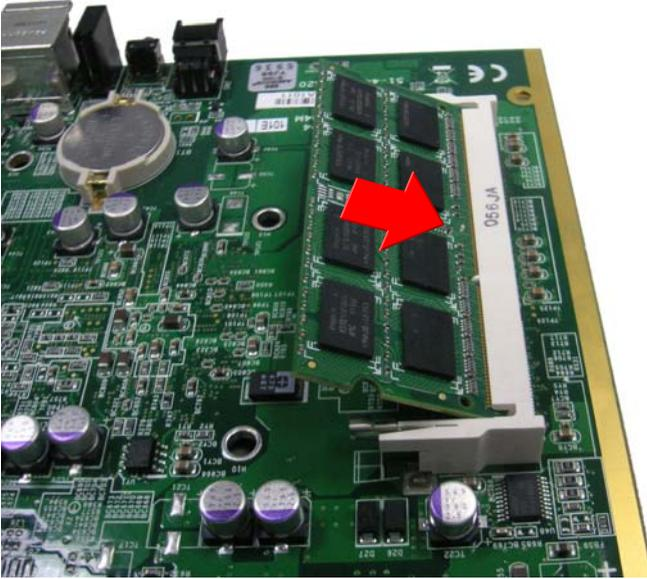
3. Depress RAM until the latch catches and the RAM is securely fixed..
