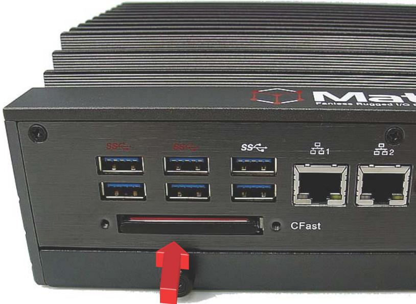
3. Re-assemble the CFast cover and fasten the 2 screws on the front panel.
