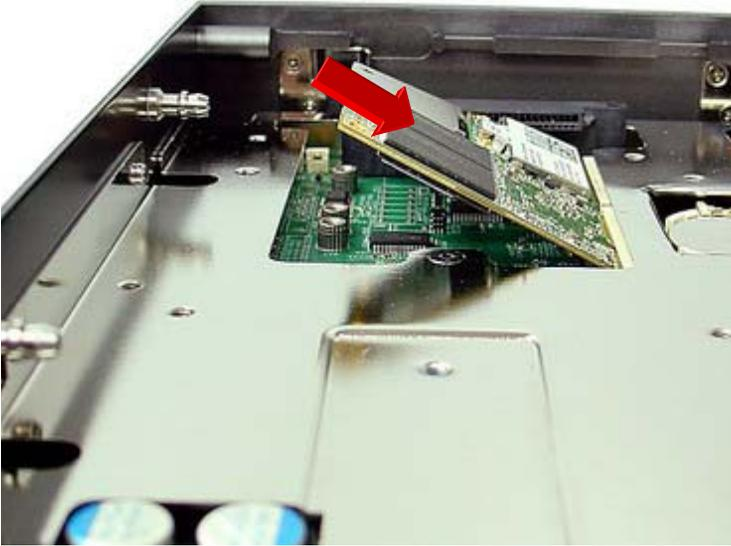
3. Depress the mini-PCIE wireless module into place and use the 2 M2.5-P-head-L5 screws to fix the module.
