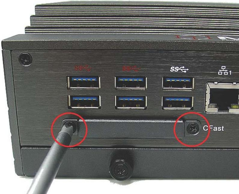
2. Gently insert the CFast card into the CFast socket.
