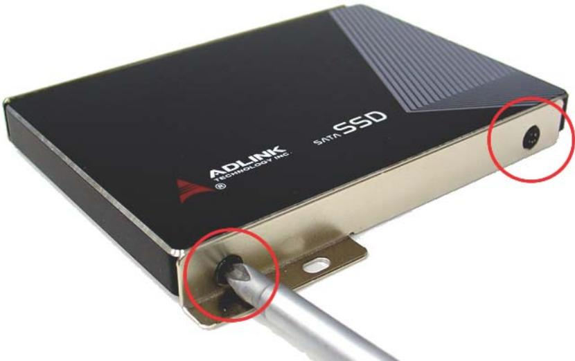
4. Install the hard disk drive and fasten the 2 M3-head-L4 screws on the top of the HDD brackets. Two hard disk drives are supported.
