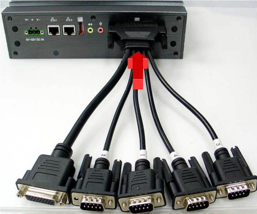
The 4 COM port cables are numbered 1 to 4, with 1 and 2 (COM1 & COM2) BIOS configurable and connecting to RS-232/422/485 devices and 3 and 4 (COM3 & 4) to RS-232 interface devices.
