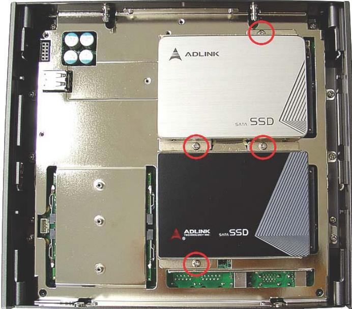
5. Re-assemble the bottom cover and fasten the thumb-screws on the front panel by hand or screwdriver.
