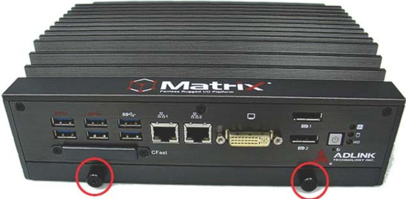
2. Withdraw the thumbscrews and remove the bottom cover by pulling and lifting.
