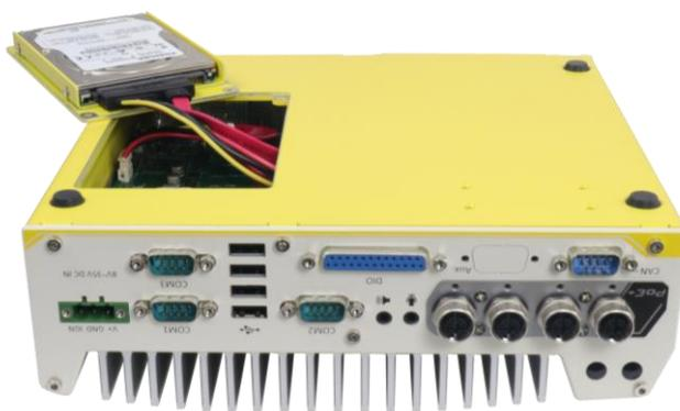
5. Gently wiggle the bracket back into the enclosure and secure it with three (3) M3 flat-head screws.
