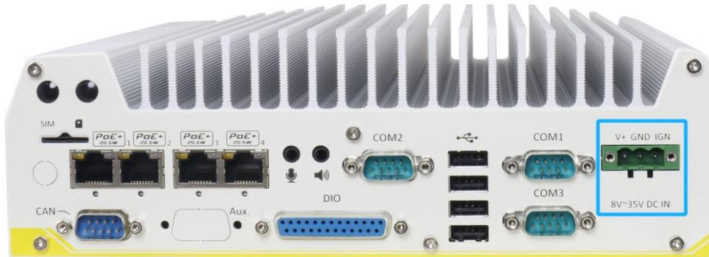
To have ignition power control for in-vehicle usage, you need to supply IGN signal to the system. The IGN input is located on the 3-pin pluggable terminal block (shared with DC power input). Below is the typical wiring configuration for in-vehicle applications.
