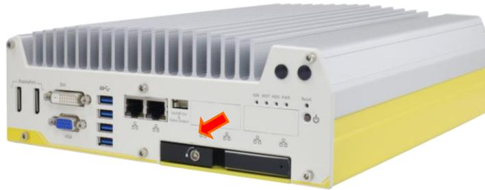
3. With HDD/ SSD label facing upwards, insert the gold finger end of the 2.5" HDD/SSD into the tray.
