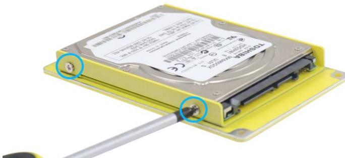
4. Connect the SATA cable inside the enclosure to the HDD/ SSD
