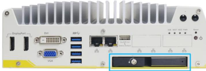
2. Pull the handle of the tray door to open the hot-swappable HDD tray.
