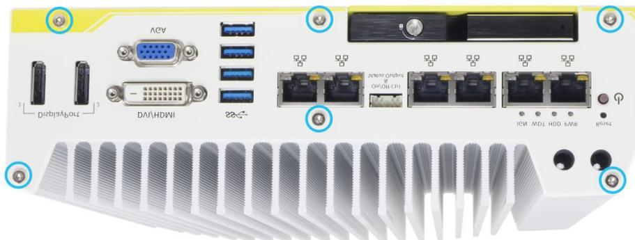
3. On the rear panel, remove the six (6) screws indicated.
