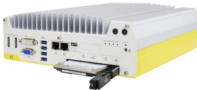
4. Push the handle into the HDD tray with HDD until it snaps into position.
