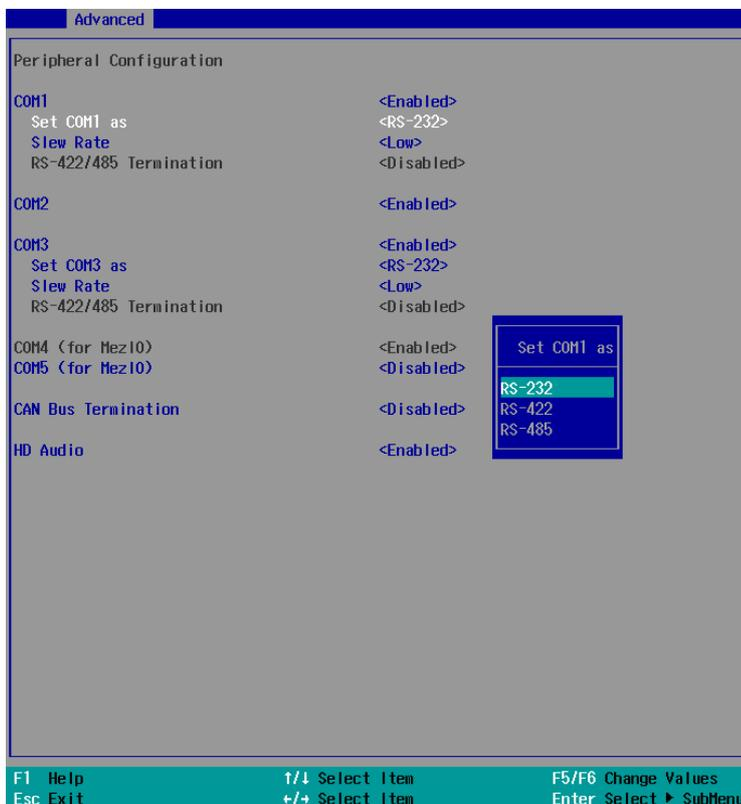
Another option in BIOS called “*Slew Rate*” defines how sharp the rising/falling edge is for the output signal of COM1/ COM3. For long-distance RS-422/485 transmission, you may set the “*Slew Rate*” option as “High” to improve signal quality.
