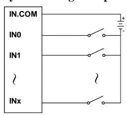
TTL/CMOS signal Input
