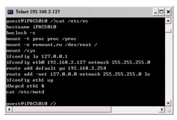
To configure the IP address, Netmask and Gateway setting, please modify /disk/etc/rc as following:
