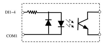
DIx: Isolated digital input channels COMx: common ground of four DIx
