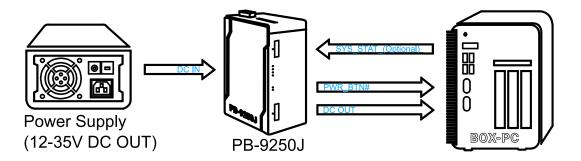
**Normal Backup Mode** is for general purpose use of PB-9250J/ 4600J. In Normal Backup Mode, DC output 12~35V from power supply should be connected to the DC IN of PB-9250J/ 4600J. DC OUT of PB-9250J/ 4600J should be connected to the power input of the back-end system. In addition, user should connect PWRBTN# signal pairs to the remote control or whichever connector that is connected to the power button signal of the back-end system.
