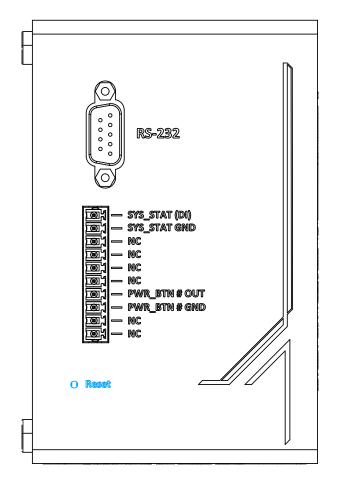
The reset button is used to manually reset and load system default configuration in case of a system halt or malfunction. To avoid unexpected operation, the button is purposely placed behind the panel. To reset the system, please use a pin to poke the button behind the panel for 5 seconds till one long beep heard.
