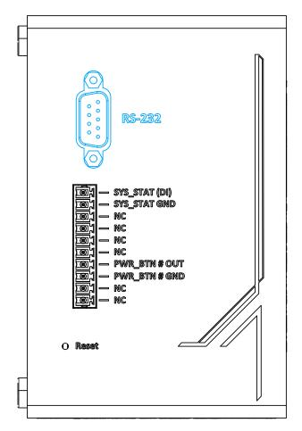
The 9-pin D-sub COM port can connect and communicate with the host computer to acquire PB-9250J/ 4600J information.
