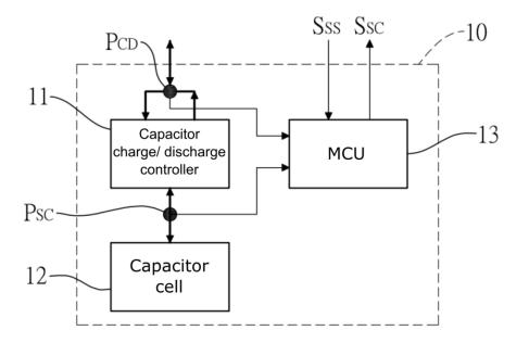
By providing sophisticated real-time energy monitoring, high/ low voltage protection and auto/ manual shutdown control, the dedicated interface help users better manage and efficiently utilize their PB-9250J/ 4600J. The software can also extend the lifespan of ultracapacitors up to 4.8x by controlling charge/ discharge cycles.
