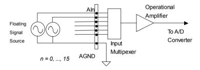
Figure 4.2.1 Floating source and single-ended
