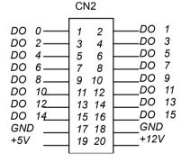
Figure 2.8.3 Pin Assignment of CN2
