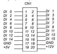
Figure 2.8.2 Pin Assignment of CN1
