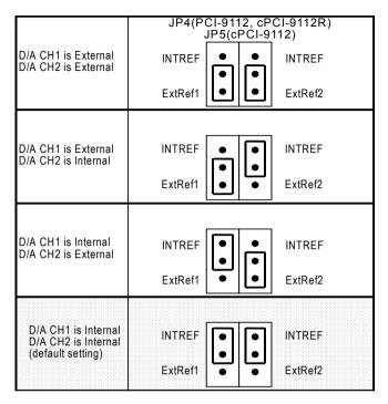
Figure 2.6 Analog Output Voltage Setting
