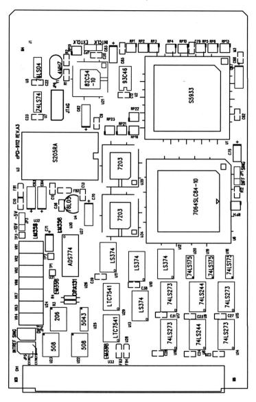
Figure 2.2 PCB Layout of the cPCI-9112
