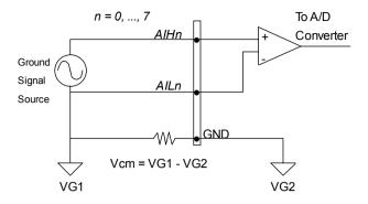
Figure 4.2.2 Ground source and differential input
