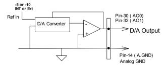
Figure 4.3 Connection of Analog Output Connection
