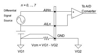
Figure 4.2.3 Differential source and differential input
