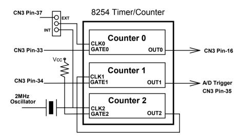
Figure 4.5 Block Diagram of 8254 Timer/Counter
