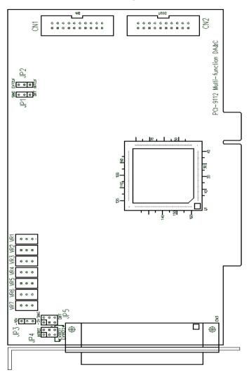
Figure 2.1 PCB Layout of the PCI-9112
