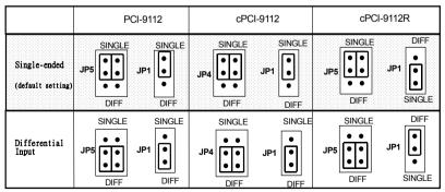
Figure 2.4 Analog Input Mode Setting
