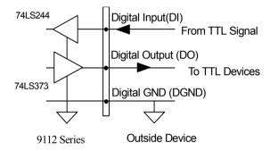
Figure 4.4 Digital I/O Connection
