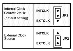
Figure 2.5 Timer's Clock Source Setting
