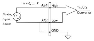
Figure 4.2.4 Floating source and differential input
