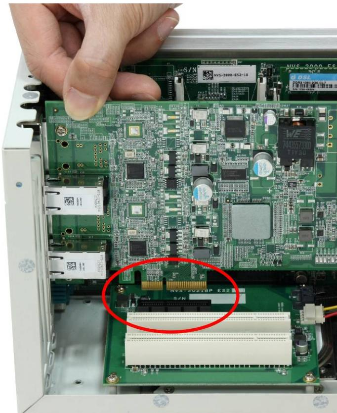
3. Fix the PCIe-PoE2+ to the host computer using with a screw.
