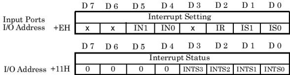
**Figure 4.15. Input Port Assignment of Interrupt Function**
