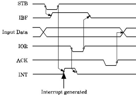
**Figure 4.14. Timing of Handshake Function**
