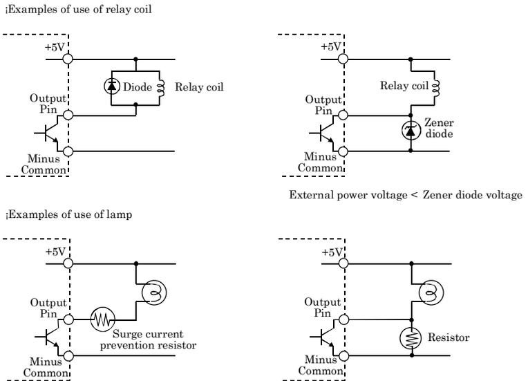
**Figure 3.10. Samples of Voltage Surge Protection**
