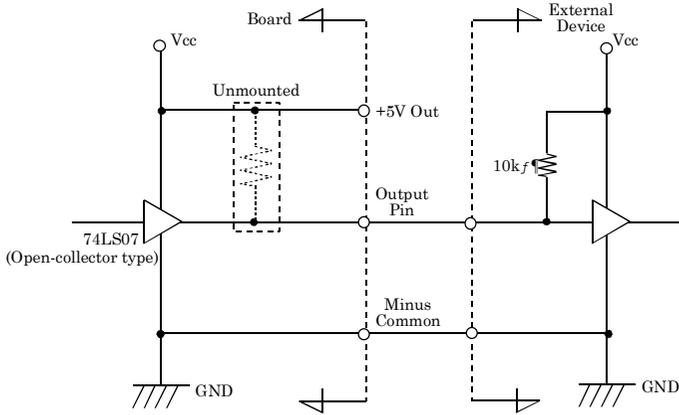
Figure 3.6. Output Circuit
