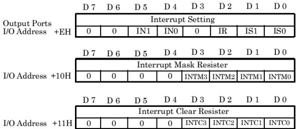
**Figure 4.16. Output Port Assignment of Interrupt Function**
