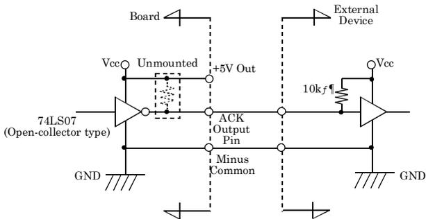
Figure 3.8. ACK Output Circuit
