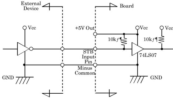
Figure 3.7. STB Input Circuit
