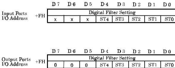
Figure 4.10. I/O Ports of Digital Filter Function
