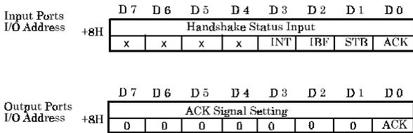
**Figure 4.13. I/O Port Assignment of Handshake Function**
