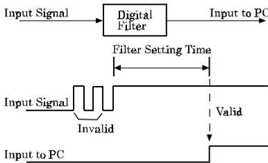
Figure 4.9. Digital Filter Operation Principle
