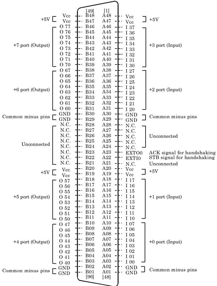
Figure 3.3. Interface Connector Pin Assignment
