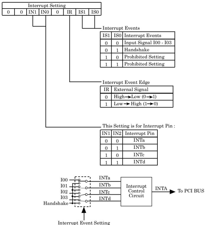
Figure 4.17. Explanation of Interrupt Setting Register
