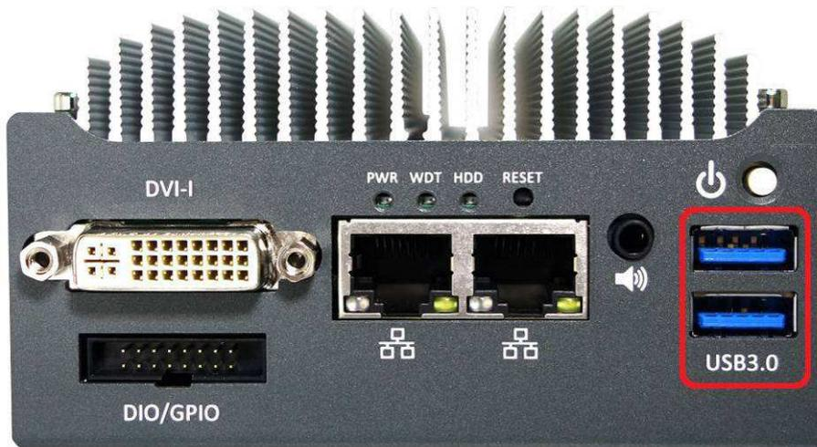
There are totally three USB 3.0 ports and one USB 2.0 port on POC-200 series. Two of three USB 3.0 ports are located on the front panel. They are implemented via a Renesas uPD720202 USB3 host controller. By BIOS default, these USB ports are operated in xHCI (eXtensible Host Control Interface) mode and are compatible to USB 3.0, USB 2.0, USB 1.1 and USB 1.0 devices. Legacy USB support on these ports is provided only when “xHCI Mode” option in BIOS is configured as “Smart Auto”.
