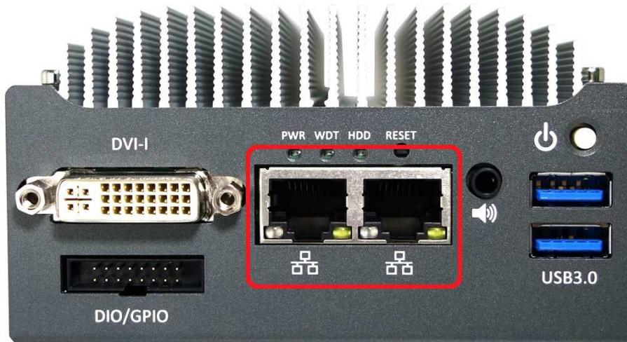
POC-200 series offers two Gigabit Ethernet ports using Intel® I210 GbE controller. When plugging in the Ethernet cable, you can tell the Ethernet status and speed from the LED indicators on the RJ45 connector as following:
