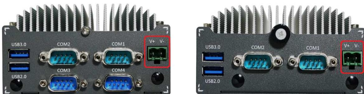
5. Push the terminal block to the power plug till it's firmly attached. Now you can supply the DC power and operate your POC-200.
