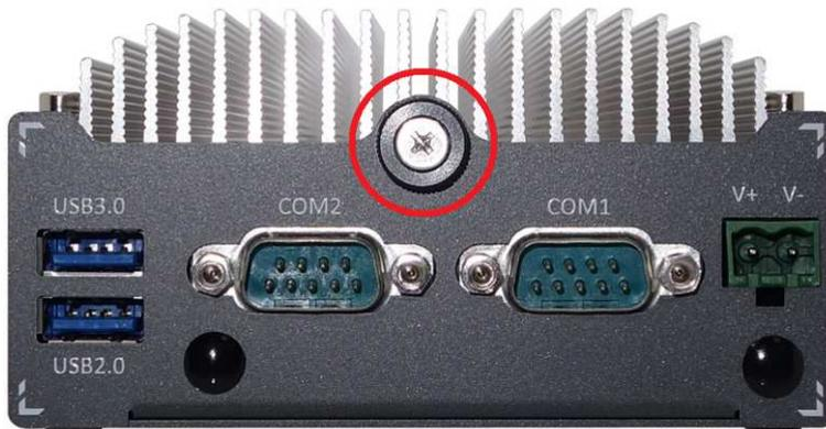
2. Pull the 2.5" HDD bracket out of POC-212/222.
