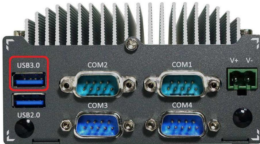
There are totally three USB 3.0 ports and one USB 2.0 port on POC-200 series. One of three USB 3.0 ports is located on the back panel. This USB 3.0 port is implemented via native xHCI controller inside Bay Trail SoC. By BIOS default, this USB port is operated in xHCI (eXtensible Host Control Interface) mode and is compatible to USB 3.0, USB 2.0, USB 1.1 and USB 1.0 devices.
