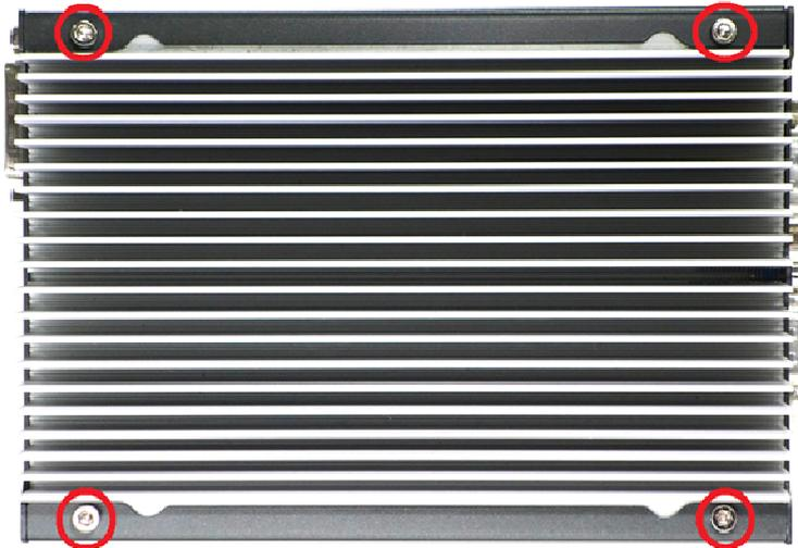
2. Unscrew four M3 F-head screws on the bottom side.
