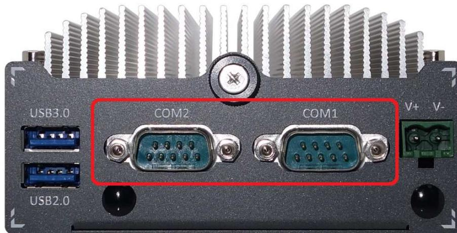
POC-212 and POC-222 provide two COM ports via two 9-pin D-Sub male connectors on the back panel for communicating with external devices. They are implemented using industrial-grade ITE8783 Super IO chip (-40 to 85°C) and provide up to 115200 bps baud rate.
