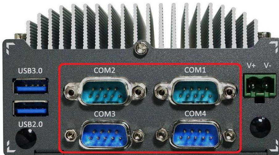
POC-200 and POC-210 provide four COM ports via four 9-pin D-Sub male connectors on the back panel for communicating with external devices. They are implemented using industrial-grade ITE8783 Super IO chip (-40 to 85°C) and provide up to 115200 bps baud rate.
