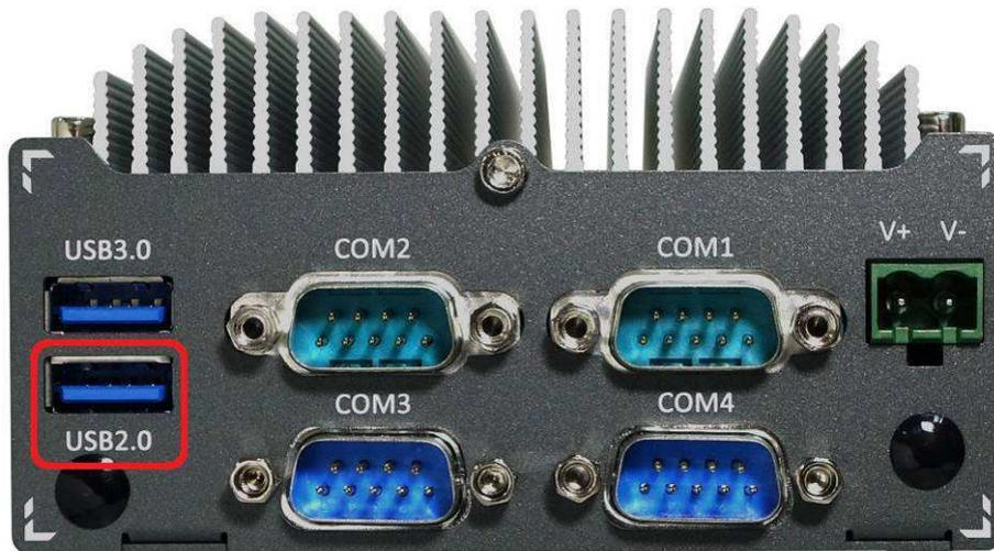
In addition to three USB 3.0 ports, POC-200 series provides another USB 2.0 port on its back panel. By BIOS default, these USB 2.0 ports are operated in EHCI (Enhanced Host Control Interface) mode and are compatible with USB 2.0, USB 1.1 and USB 1.0 devices. Legacy USB support is provided so you can use USB keyboard/mouse in DOS environment.
