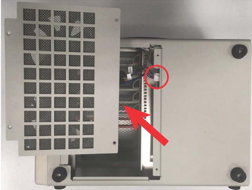
4. Withdraw the fan module from the chassis and remove the eight fixing screws.
