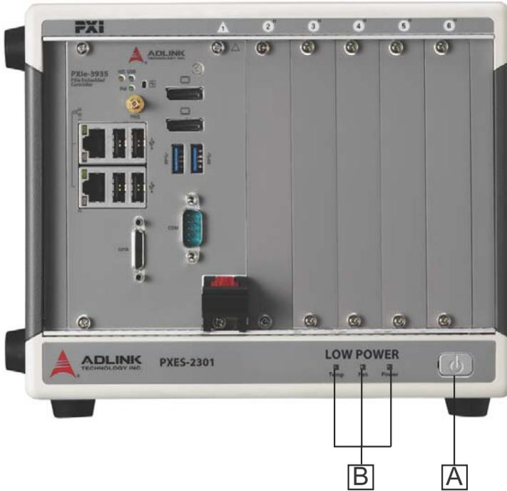
**Figure 1-7: PXES-2301 Front Panel**
