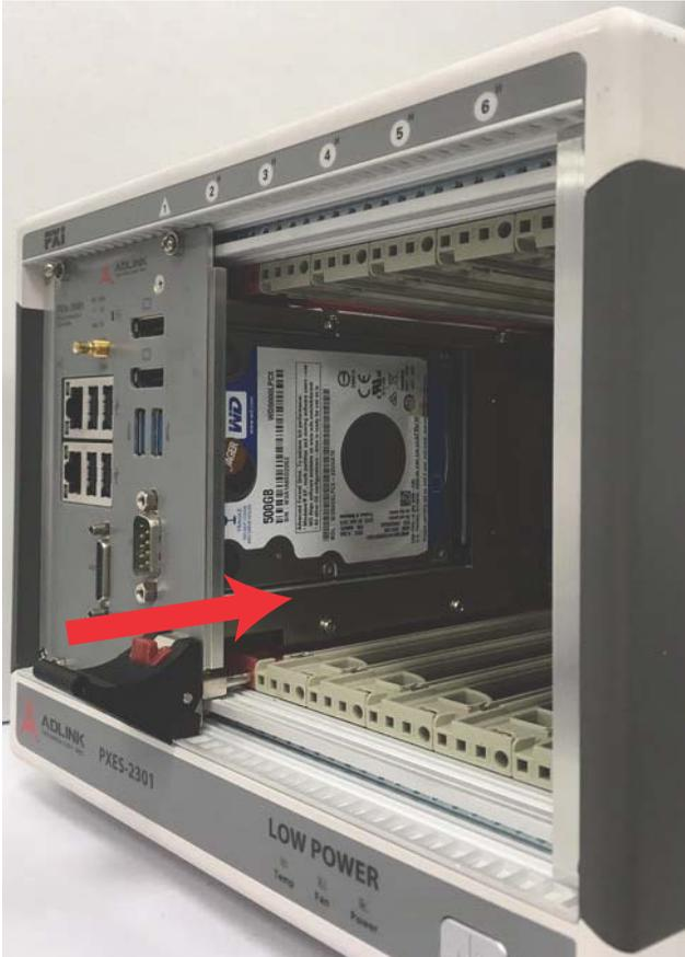
5. Lift the latch until the module is securely seated in the chassis backplane
