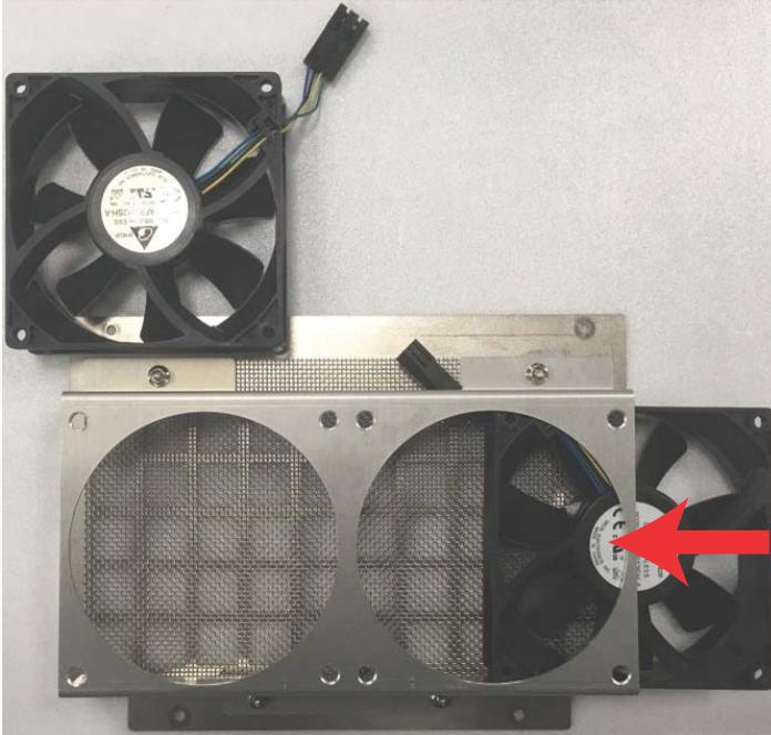
6. Replace the fixing screws and reseat the fan module in the chassis. Replace the cover.
