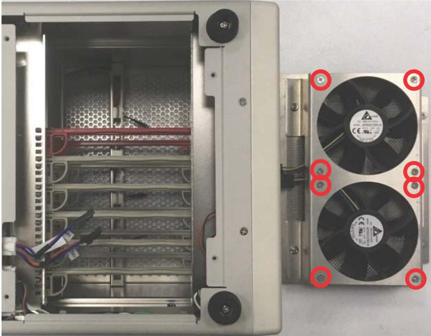
5. Remove the two cooling fan units from the module and replace with new units.
