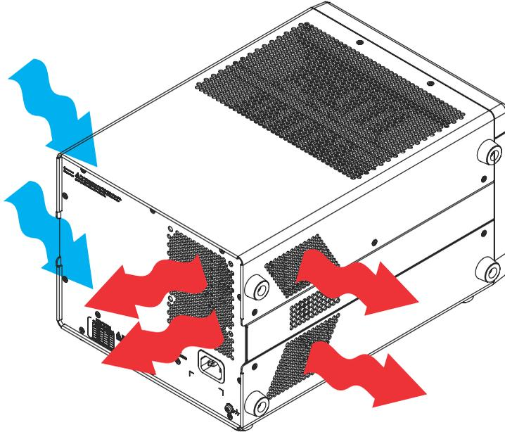
The PXES-2780 should be situated on a bench top or in an instrument rack, maintaining at least 1U (44.5 mm/1.75 in.) clearance from all ventilation apertures. Further, the 12.7mm/0.5 in. height of the rubber feet on the underside must be maintained to allow air intake.
