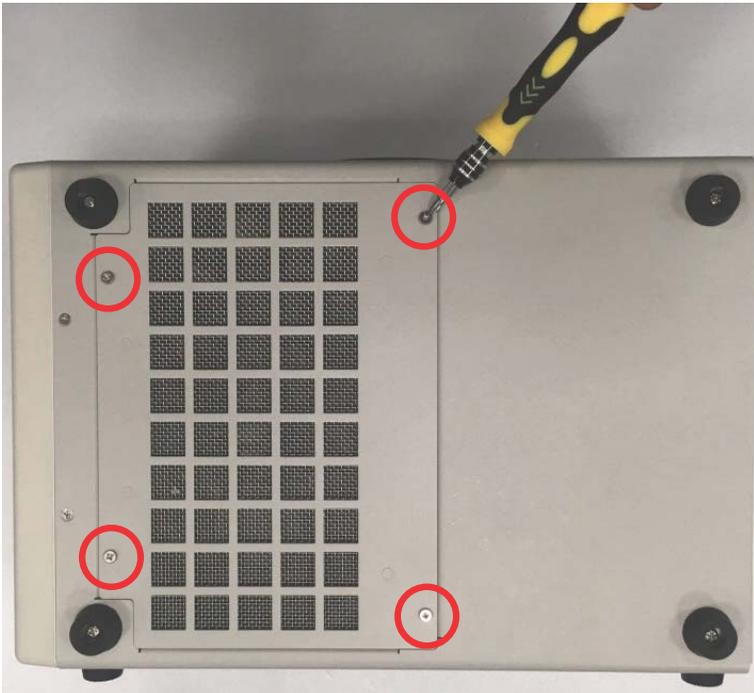
3. Remove the fan module cover and detach the two cable harnesses connected to the backplane.
