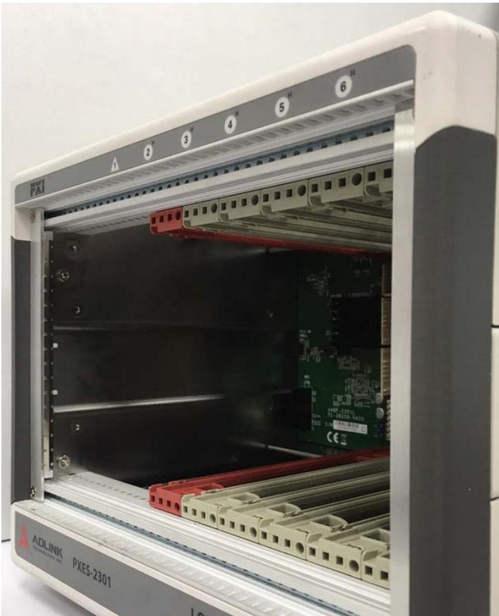
3. Depress the system controller module's latch to release.
