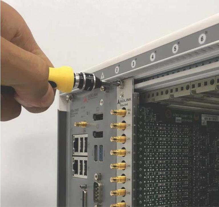
6. Repeat steps 1 to 5 to install additional PXI or PXES peripheral modules.
