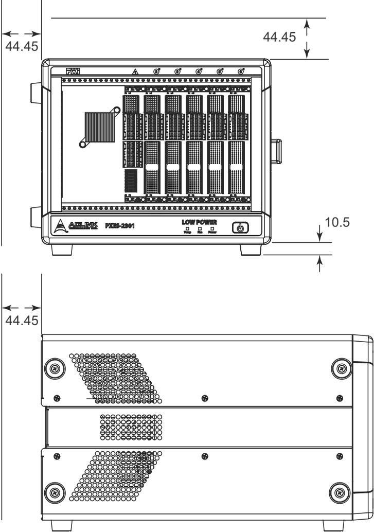
Figure 2-1: Cooling Clearances
