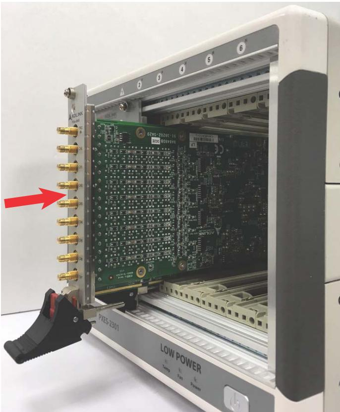
5. Fasten the screws on the module's front panel.
