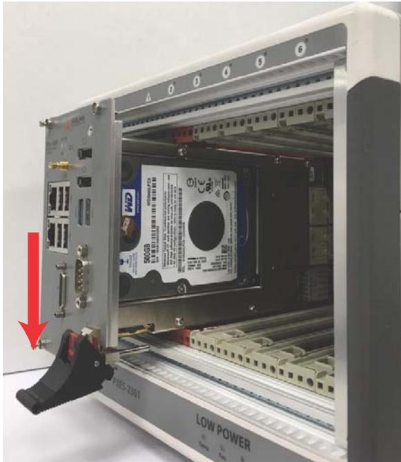
4. Align the module's top and bottom edges with the card guides, and carefully slide the module into the chassis.
