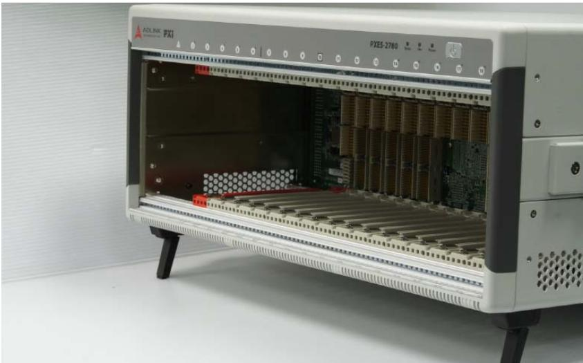
3. Depress the system controller module's latch to release.
