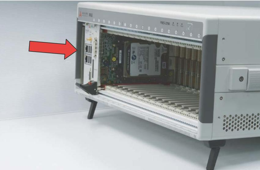
5. Lift the latch until the module is securely seated in the chassis backplane
