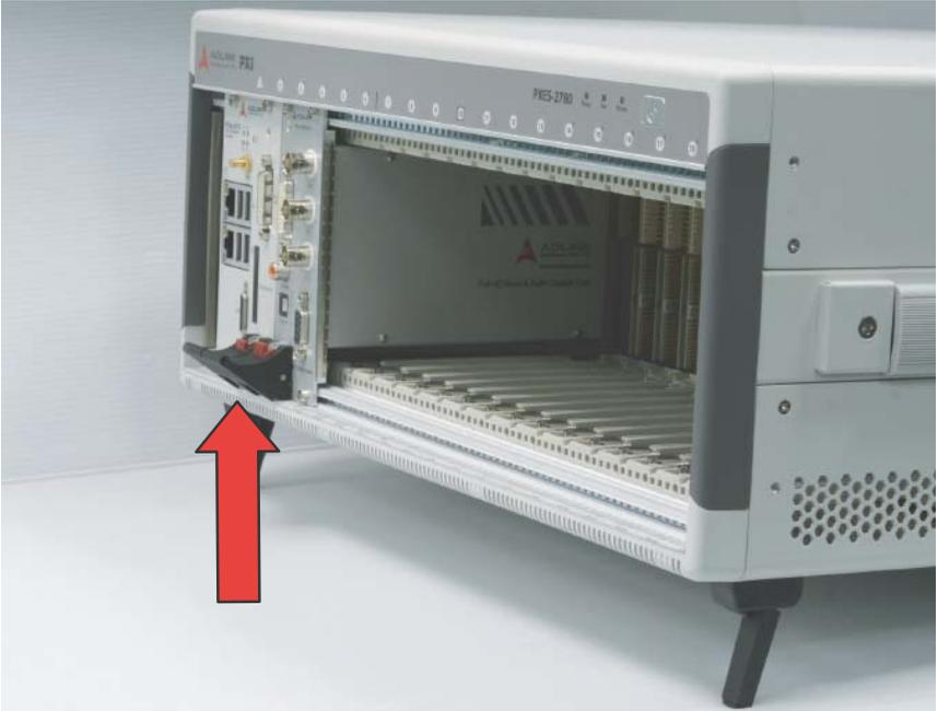
5. Fasten the screws on the module's front panel.
