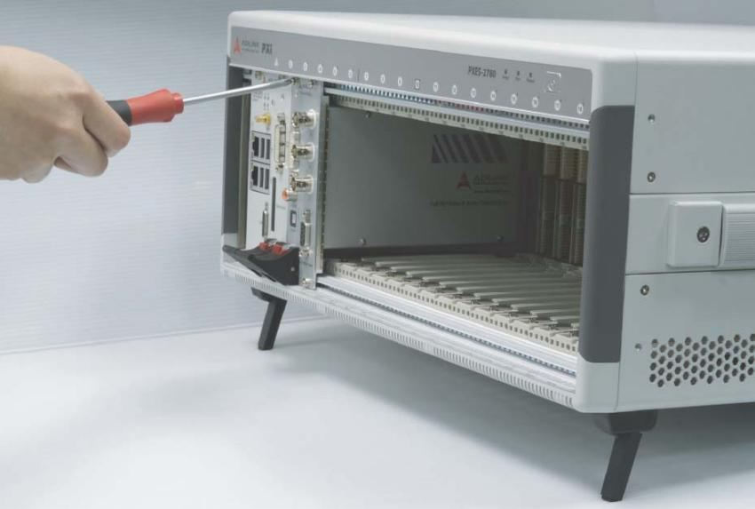
6. Repeat steps 1 to 5 to install additional PXI orPXIe peripheral modules.
