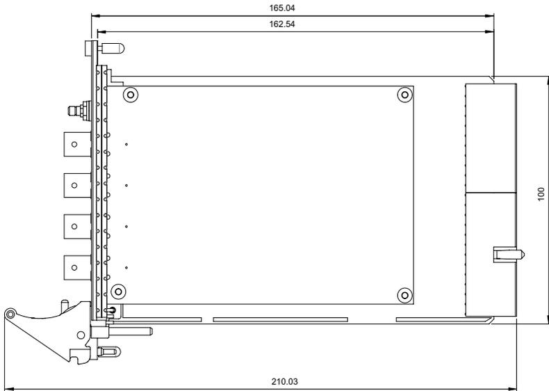
**Figure 2-1: PXI-9527 Side View**
