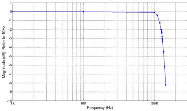
**Figure 1-1: Analog Input Channel Bandwidth,  $\pm 10$  V Input Range**
