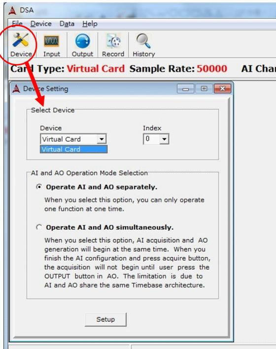
Figure 1-3: DSA Device Setting Interface
