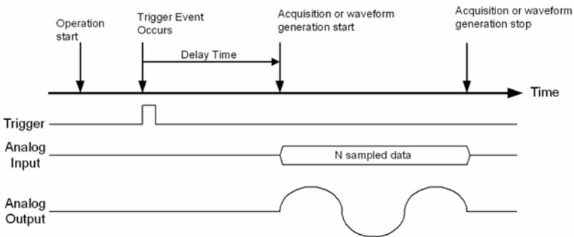
**Figure 3-8: Delay Trigger Mode Acquisition / Waveform Generation**
