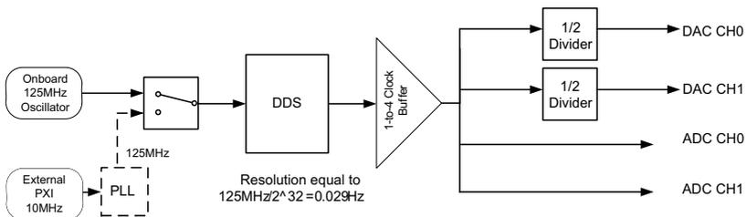
**Figure 3-9: PXI-9527 Timebase Architecture**
