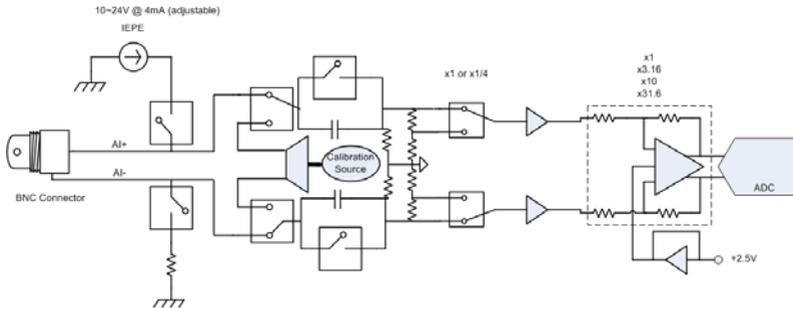
**Figure 3-1: Analog Input Architecture of the PXI-9527**
