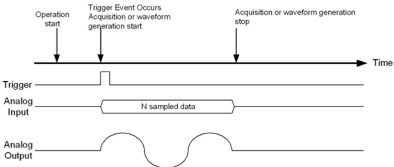
**Figure 3-7: Post-trigger Acquisition / Waveform Generation**
