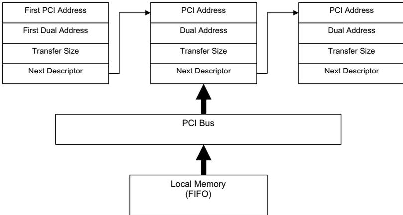
Figure 3-2: Linked List of PCI Address DMA Descriptors
