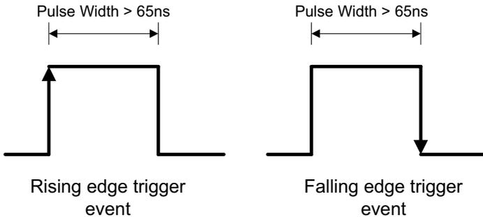
**Figure 3-5: External Digital Trigger**
