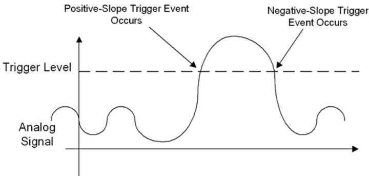
**Figure 3-6: Analog Trigger Conditions**
