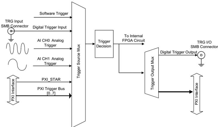
**Figure 3-4: Trigger Architecture of the PXI-9527**
