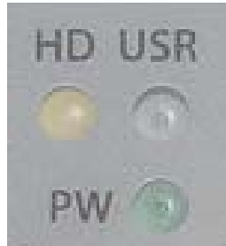
Figure 1-5: PXIe-3985 LED Indicators
