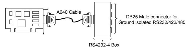
Special usage : A401 Cable or P486 Cable to connect with RS4232-4 Box. Support any RS232 device to have ground isolated RS232/RS422/RS485 interface.
