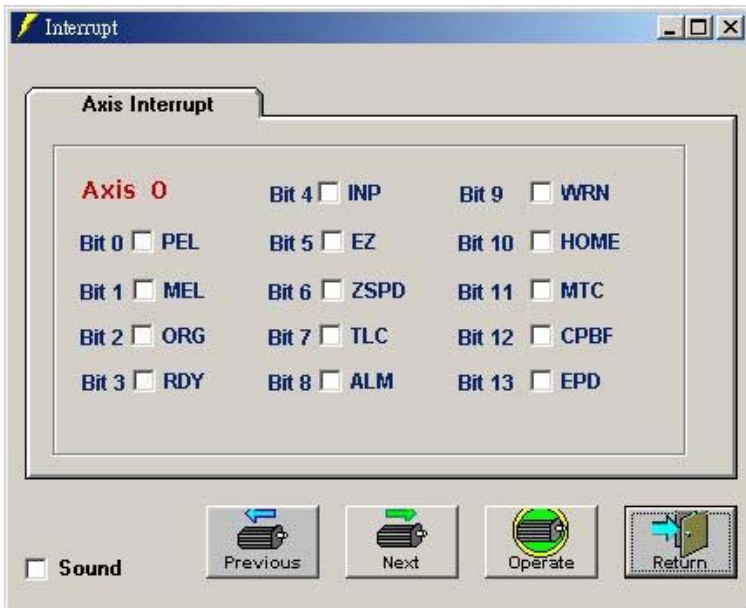
Figure 5-23: Interrupt Configuration Window
