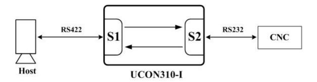
We can use UCON310-I box as RS485 to GROUND isolated **RS232 interface converter**. So we will set serial port 1 in RS485 interface type (DIP Switch bit 1 in OFF location and bit 2 set in ON location) and serial port 2 in RS232 interface type (DIP Switch bit 3 in OFF location and bit 4 in OFF location). Now we can let one RS485 device to be connected with RS232 device safety.
