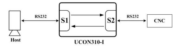
We can use UCON301-I box as **full-duplex RS422** to GROUND isolated **RS232** interface **converter**. So we will set serial port 1 in RS422 interface type (DIP Switch bit 1 and bit 2 set in ON location) and serial port 2 in RS232 interface type (DIP
