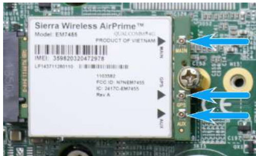
Clip on the IPEX-to-SMA cable
