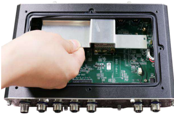
Place heatsink back on the modules
