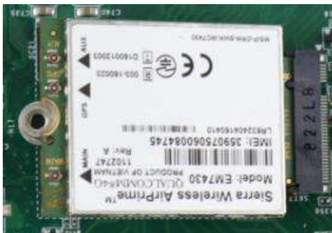
Insert on a 45° angle
