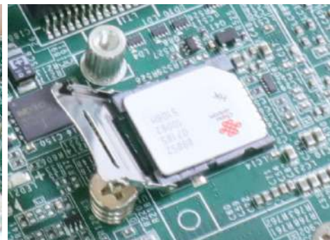
Flip open the holder and place SIM
