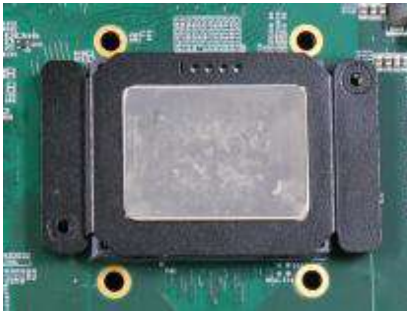
CPU retention bracket (holder)
