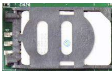
Slide and lift SIM card holder
