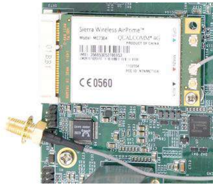
Clip on IPEX-to-SMA cable
