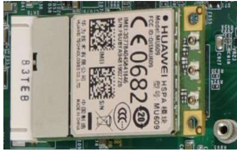
Insert on 45 degree angle
