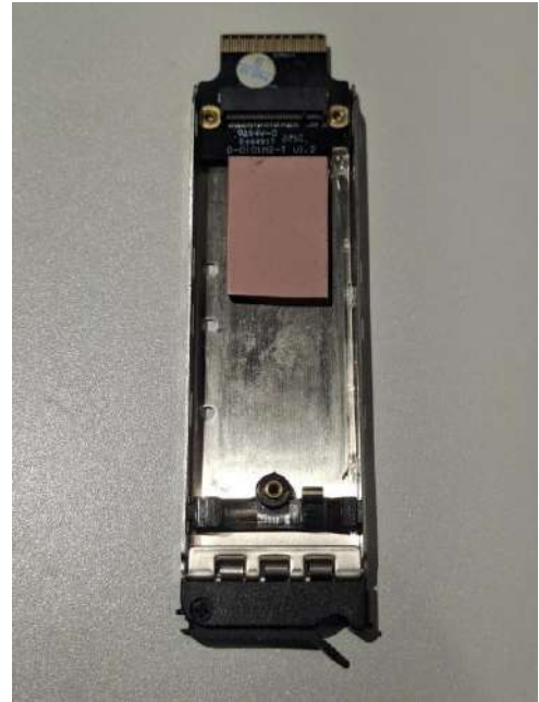
Replace with 4mm thermal pad
