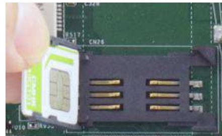
Insert SIM card with pins facing up
