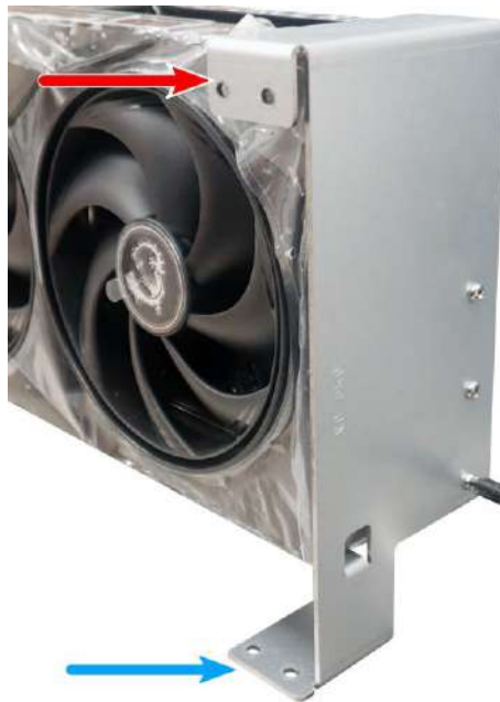
Top/ bottom screw hole to mount
