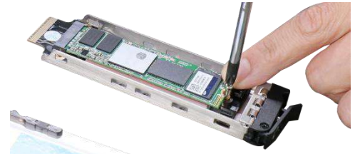
Secure with a screw
