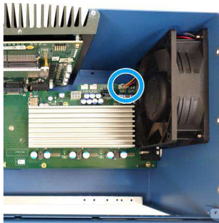
Connect the 4-pin cable
