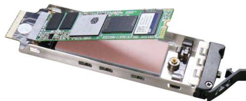
Insert on a 45° angle
