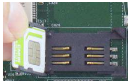
Insert SIM card with pins facing up
