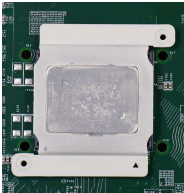
CPU retention bracket (holder)
