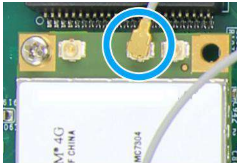
Clip on IPEX-to-SMA cable
