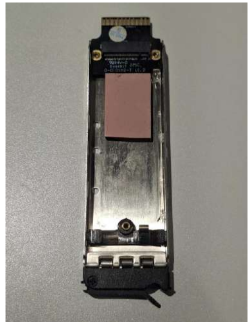
Replace with 4mm thermal pad
