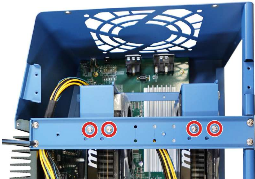
Securing RTX 50 series GPU brackets to the chassis bracket
