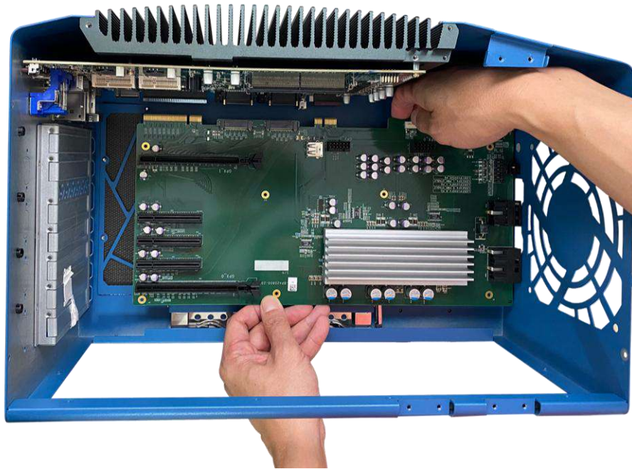
Disengage the daughter-board from the motherboard
