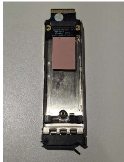
Replace with 4mm thermal pad
