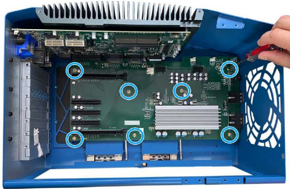
Remove screws securing the daughter-board
