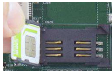
Insert Mini-SIM card with pins facing up
