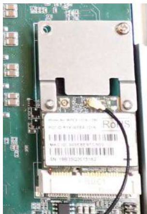
Clip on IPEX-to-SMA cable
