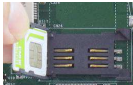
Insert Mini-SIM card with pins facing up
