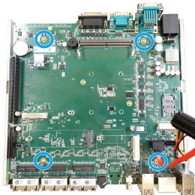
Four standoffs on the heatsink
