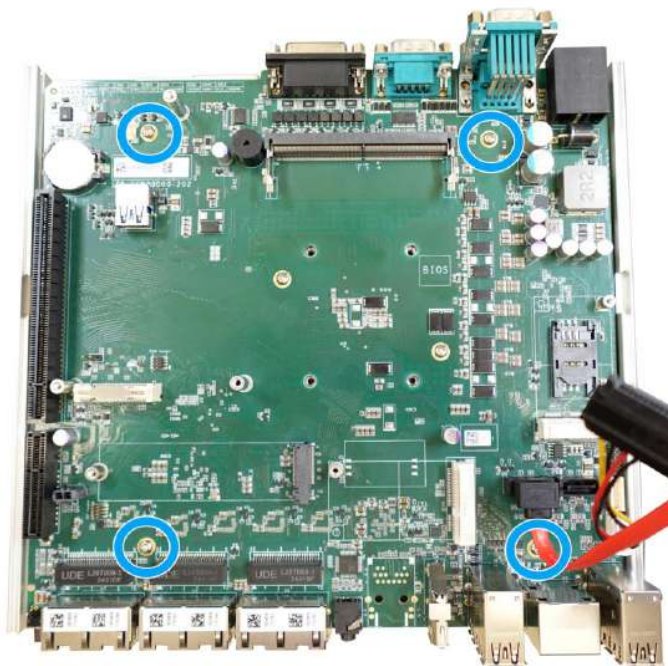
Secure motherboard with four screws
