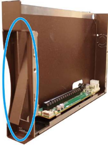
Remove bezel cover and insert the card
