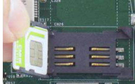
Insert Mini-SIM card with pins facing up
