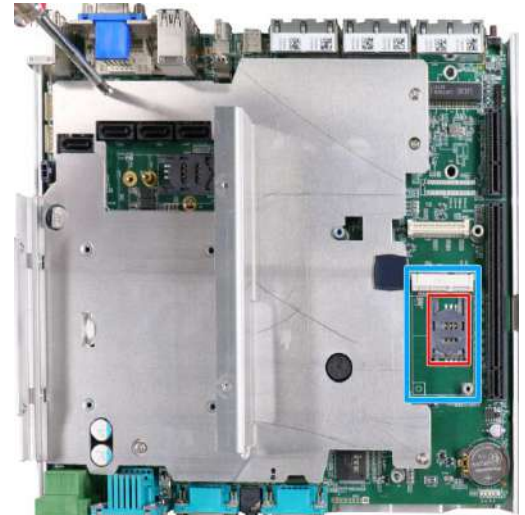
mini-PCIe slot on motherboard (underneath MezIO™ card)
