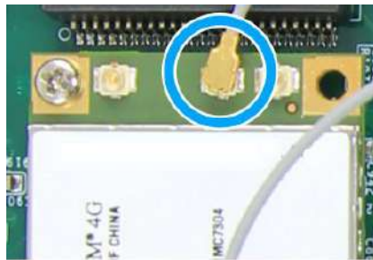
Clip on IPEX-to-SMA cable
