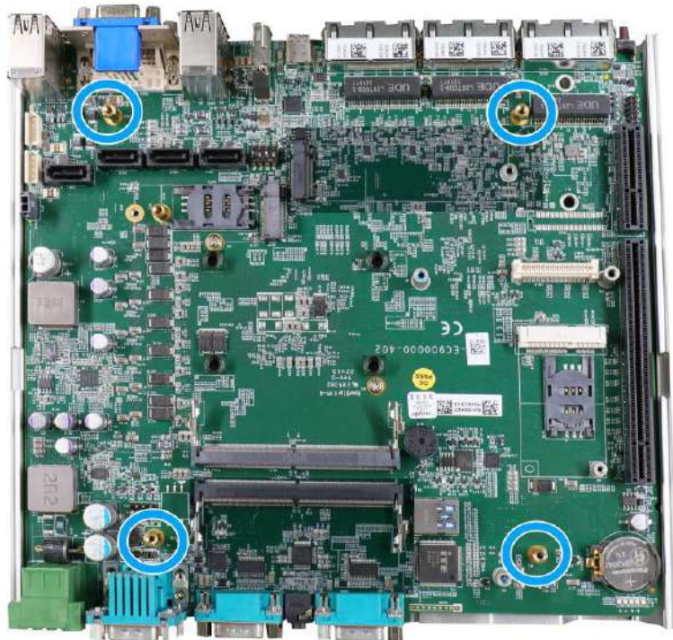
Secure motherboard with four screws
