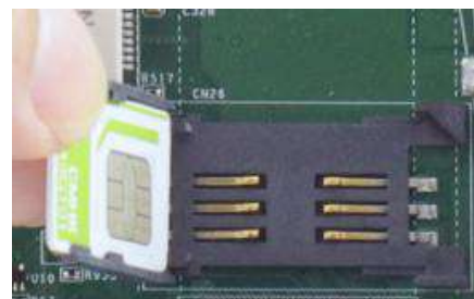
Insert Mini-SIM card with pins facing up
