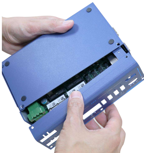
Remove front IO panel
