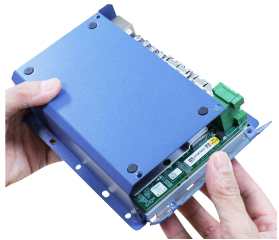
Remove reserved punch-out panel
