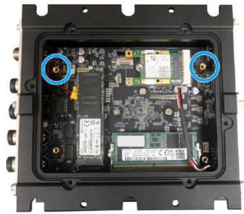
Install the copper stand-offs
