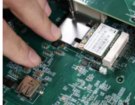
Secure the module with a screw
