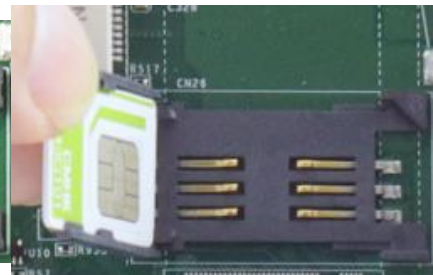
Insert SIM card with pins facing up
