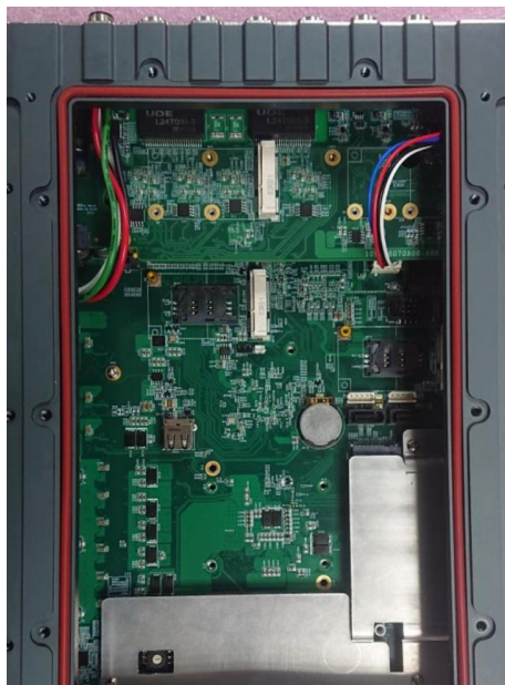
O-ring seated properly in the groove
