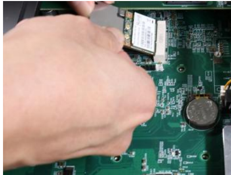
Insert into slot on a 45 degree angle
